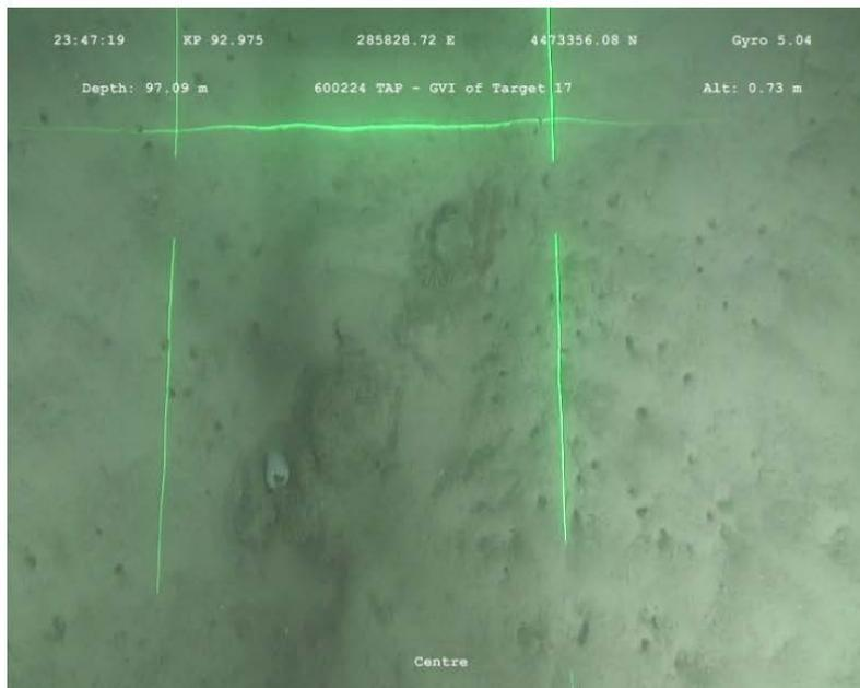
Figure 3.6 Target 017 - Magnetic anomaly 2.0m x 0.4m
