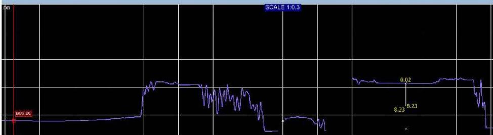
3.5 Crossprofile Cargo Hold. Height from seabed to lower deck is approximately 8m.
