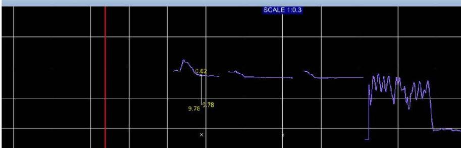
3.6 Crossprofile. Height from seabed to top of end structure is approximately 10m.
