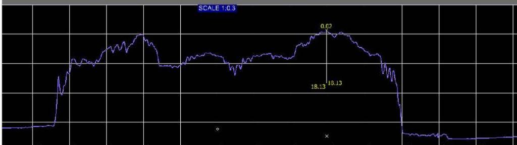
**3.4 Crossprofile midship. Height from seabed to top of structure is approximately 18m.**
