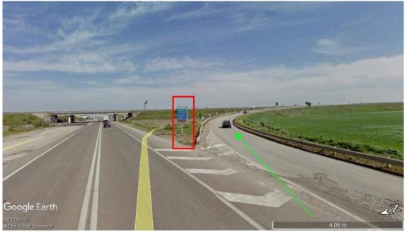
Remove the Road Signs and Black & White Chevrons from the outer radius of the curve so that the Blades can oversail the Safety Barriers.
