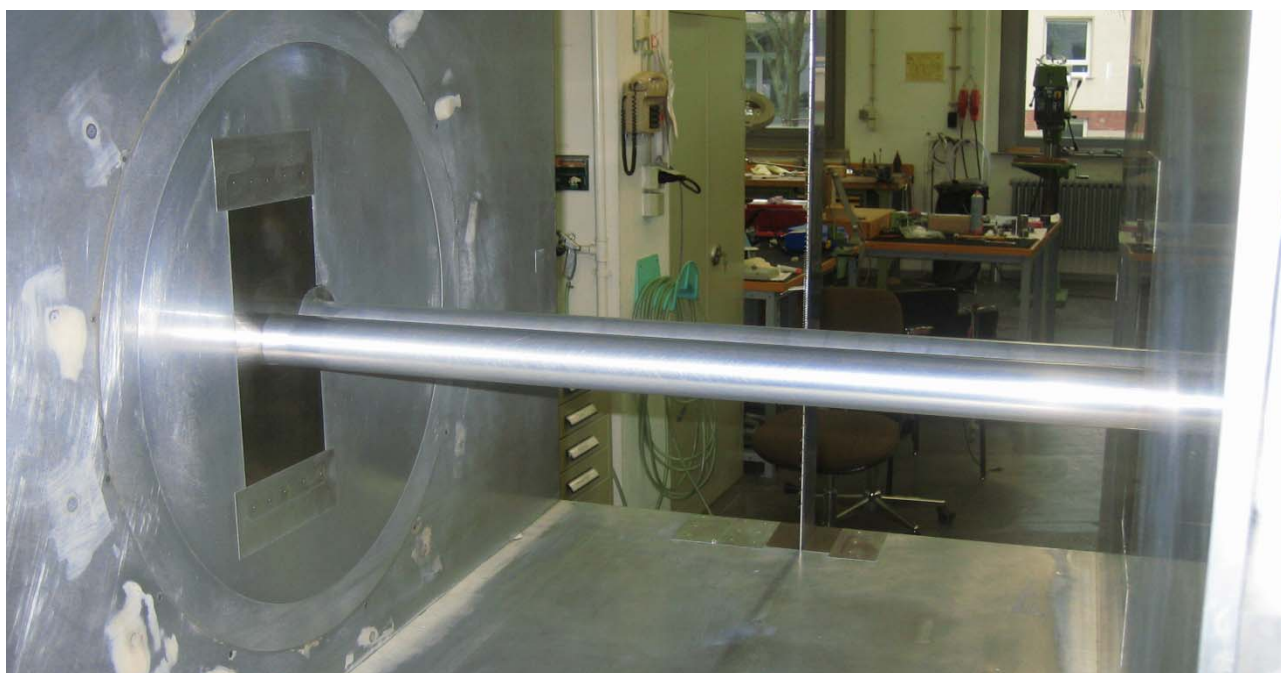
Figure 2.1 Twin cylinder model of main cable set-up in the DLR pressurized wind tunnel.
