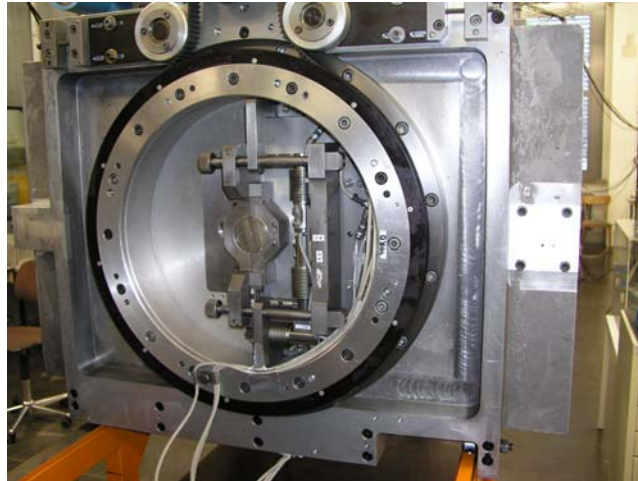
Figure 5 a: Photo of the test section, the turn table and the balance. In the centre there is the clamped cylinder under test. The three force transducer can be recognized by its bellows.
