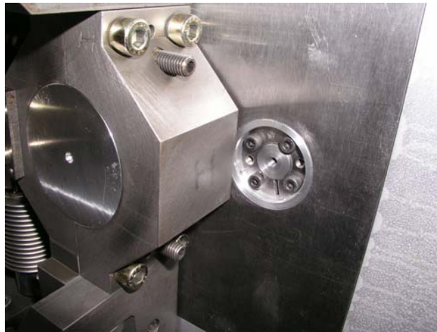
Figure 5 b: The second cylinder is attached in holes of the walls by clamping collars.
