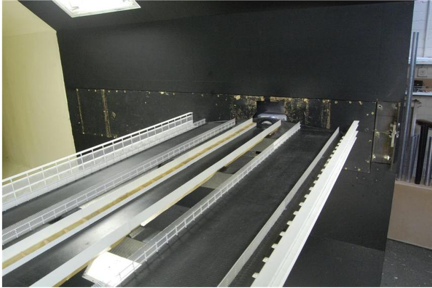
**Figure B.2: Wind Tunnel Model – Close up View of the Wind Barriers**
