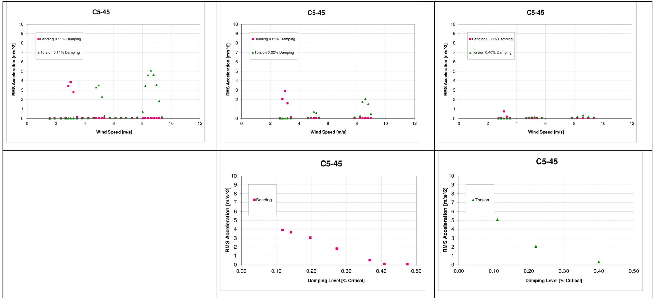
Figure 2.4 Config C5/63– Variation of MS RMS Acceleration with MS Wind Speed for Various Levels of Damping & Variation of RMS Acceleration with damping at 3ms<sup>-1</sup>
