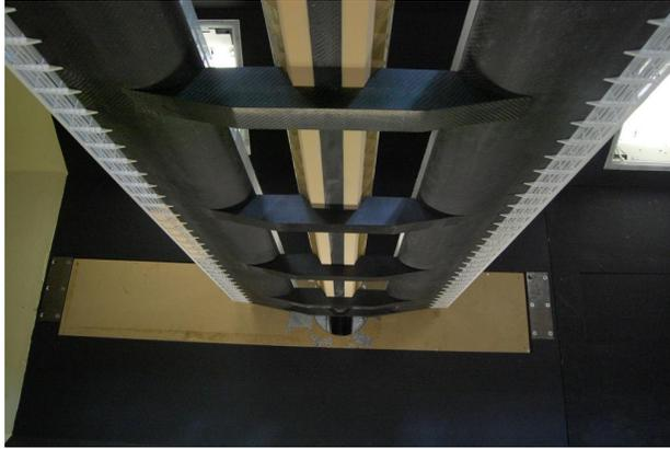
**Figure B.6: Wind Tunnel Model - Close-Up View of Underside of Model C5/63 with mesh added**
