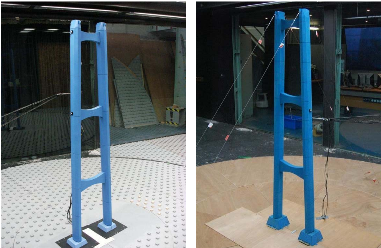
Figure 4 Full aeroelastic model prior to the tests at BMT, left side reflecting a freestanding tower, right side reflecting in service tower with pinned at the top.
