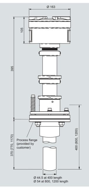
Cross-duct sensor CD 6, increased purging (instrument air), version according to Order No. 7MB6122-\*\*E1\*-0\*\*\*, dimensions in mm
