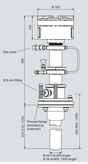
Cross-duct sensor CD 6, sensor and process side purging, version according to Order No. 7MB6122.\*\*H1\*-0\*\*\*, dimensions in mm
