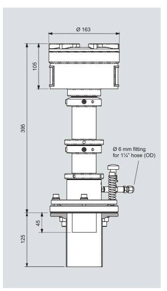
Cross-duct sensor CD 6, purged version for application SCR\_DeNOx/automotive, version according to Order No. 7MB6122-\*WC14-2\*\*\*, dimensions in mm
