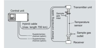
Typical transmitted light setup of LDS 6, in bypass
