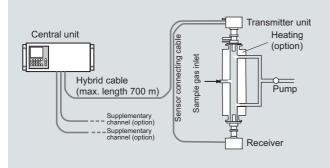
Measuring configuration of LDS 6 with heated flow cell
