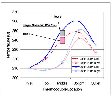
Figure 2.2-3 - SuperClaus Temperature Profile
