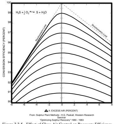
Figure 2.2-5 - Effect of Claus Air Control on Recovery Efficiency
