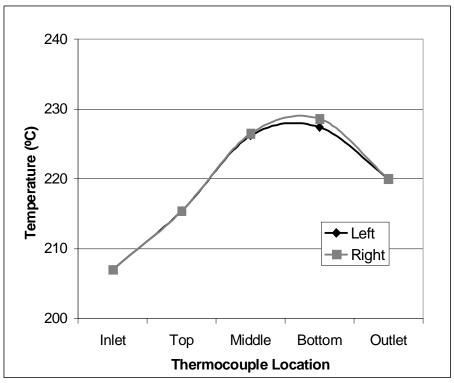
Figure 2.2-2 - ENI Gela Reactor 2 Temperature Profile
