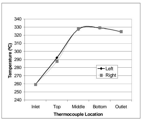
Figure 2.2-1 - ENI Gela Reactor 1 Temperature Profile
