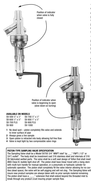
\*Also available with Flanged, or SW inlet and outlet connection. For other Sampling Valve Models refer to the size tables
