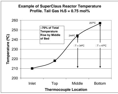
Figure E.1-1 - Ideal SuperClaus Reactor Temperature Profile
