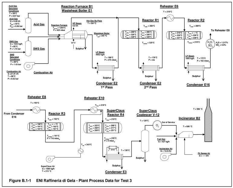
Figure B.1-1 - Plant Process Data - Test 3
