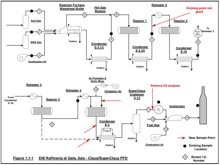
Figure 1.1-1 - Claus / SuperClaus Process Flow Diagram
