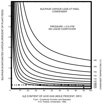
Figure 2.2-4 - Sulphur Vapour Loss At Final Condenser
