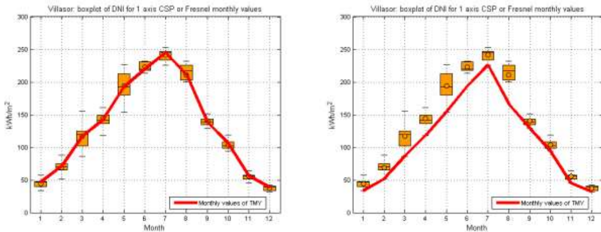
Figure 5: monthly boxplot for the driver component (1-axis tracking) (P50 on the left hand side, P90 on the right hand side)
